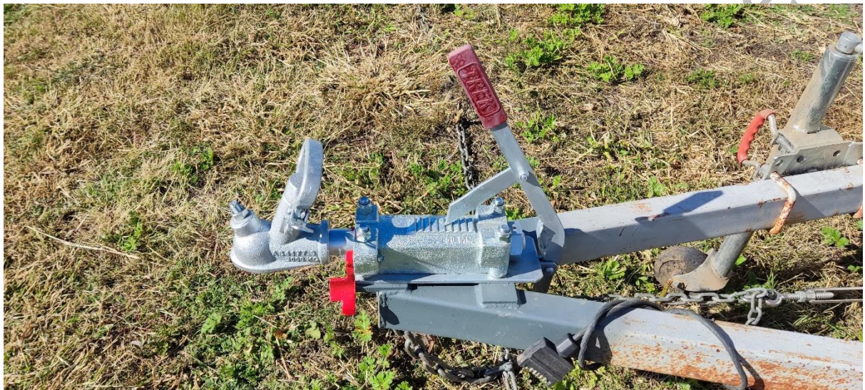
Figure 2- Handbrake applied to trailer
