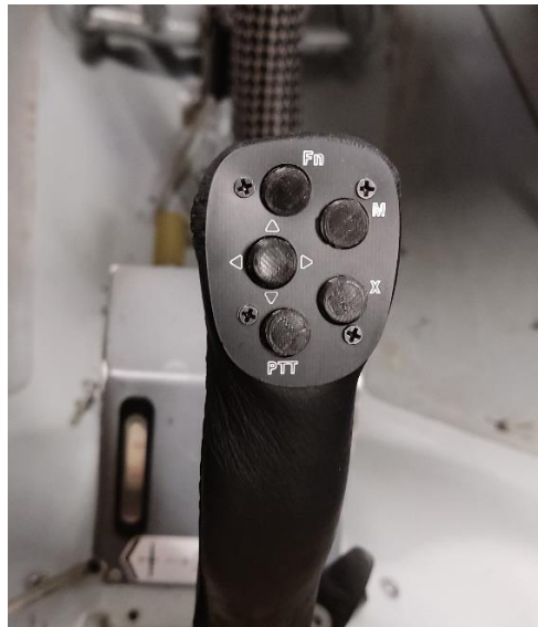
4 x pushbuttons and thumb-joystick (described above)
