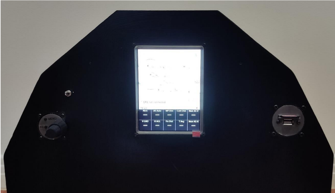
OpenVario ground training rig (note – photo shows SD card in slot on RHS of Panel. This is no longer fitted/used)
