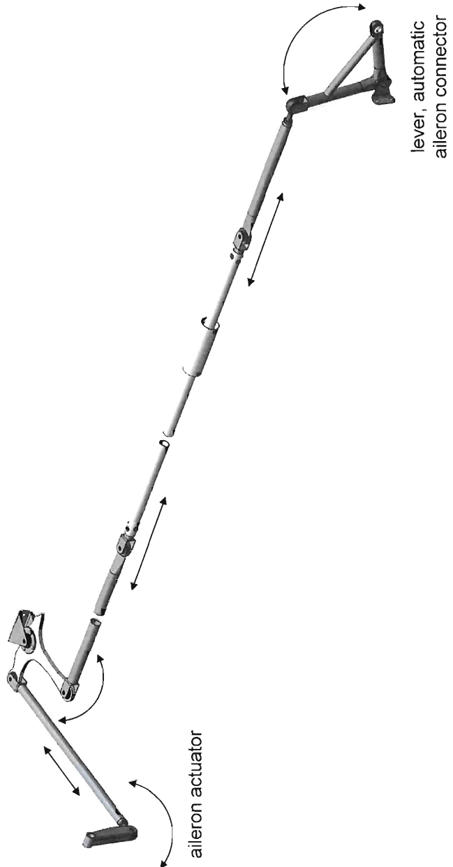
Fig. 2.2-5 Aileron Control System, Wing
