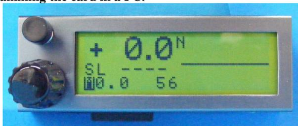
In both climb and cruise the dotted line is the current 20 second average value, TE variometer in climb, Netto in cruise.
