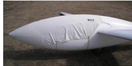
with one wing down place some protective carpet and a wing weight on the lowered wingtip and remove the tail dolly to prevent the glider shifting in windy conditions. Always install the pitot cover during storage to prevent blockage from insects such as mud wasps.
