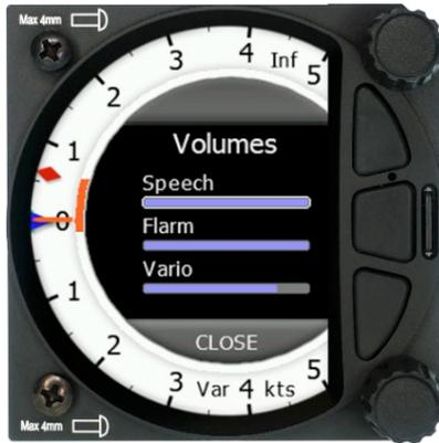
The lower rotary knob is used to adjust settings within the current mode or within menus. With the lower rotary push button, it is possible to toggle between the MC and the Ballast and Bugs settings. In all other menus this knob is used for setting values and editing texts
