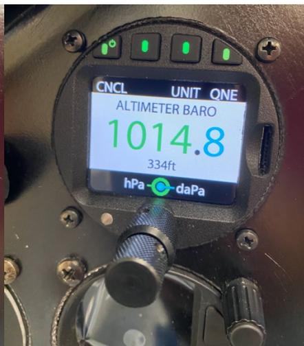
Figure 7 - altimeter Baro adjust screen
