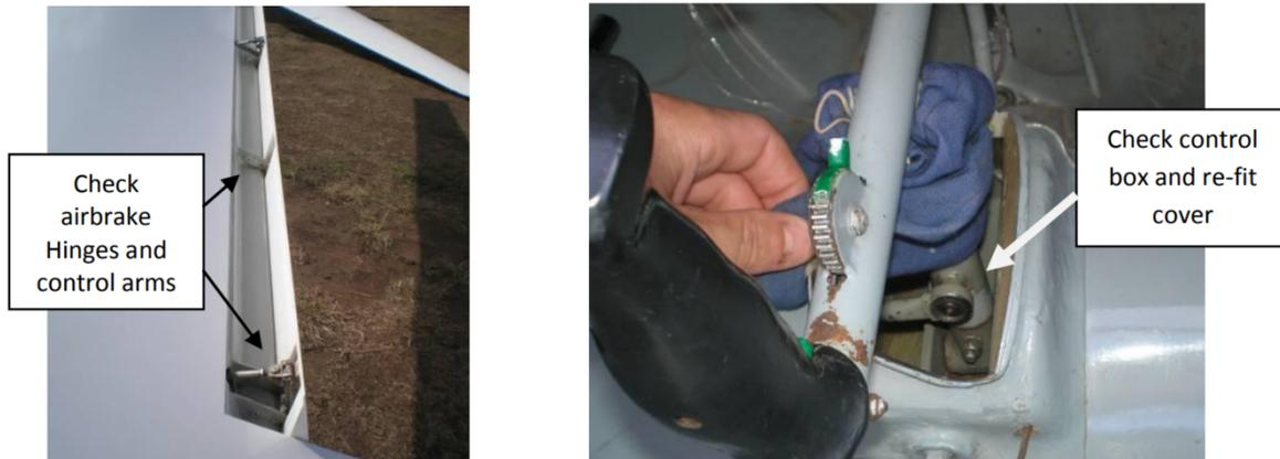
Figure 3 inspection of brakes and control box
