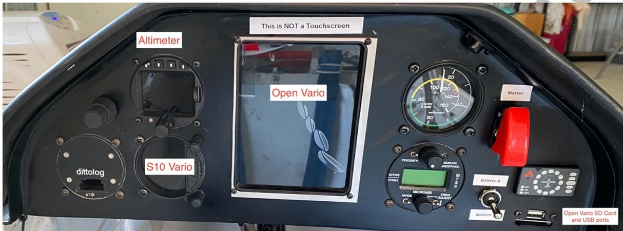
Figure 4- Instrument panel
