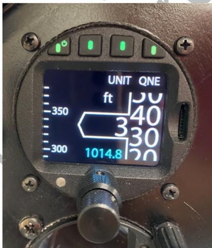
Figure 6 - altimeter main screen
