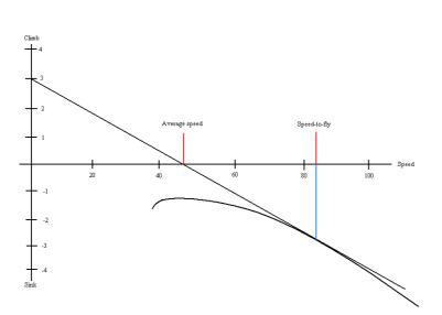
speed for the day. Again, this is for a typical ballasted 15 metre glider. Take the published polar out of your manual, (add just a small grain of salt) and plot such a graph. You may wish to write up a table of cruising speeds for given climb rates, and stick it on your panel. You will of course, remember that these speeds are really...
