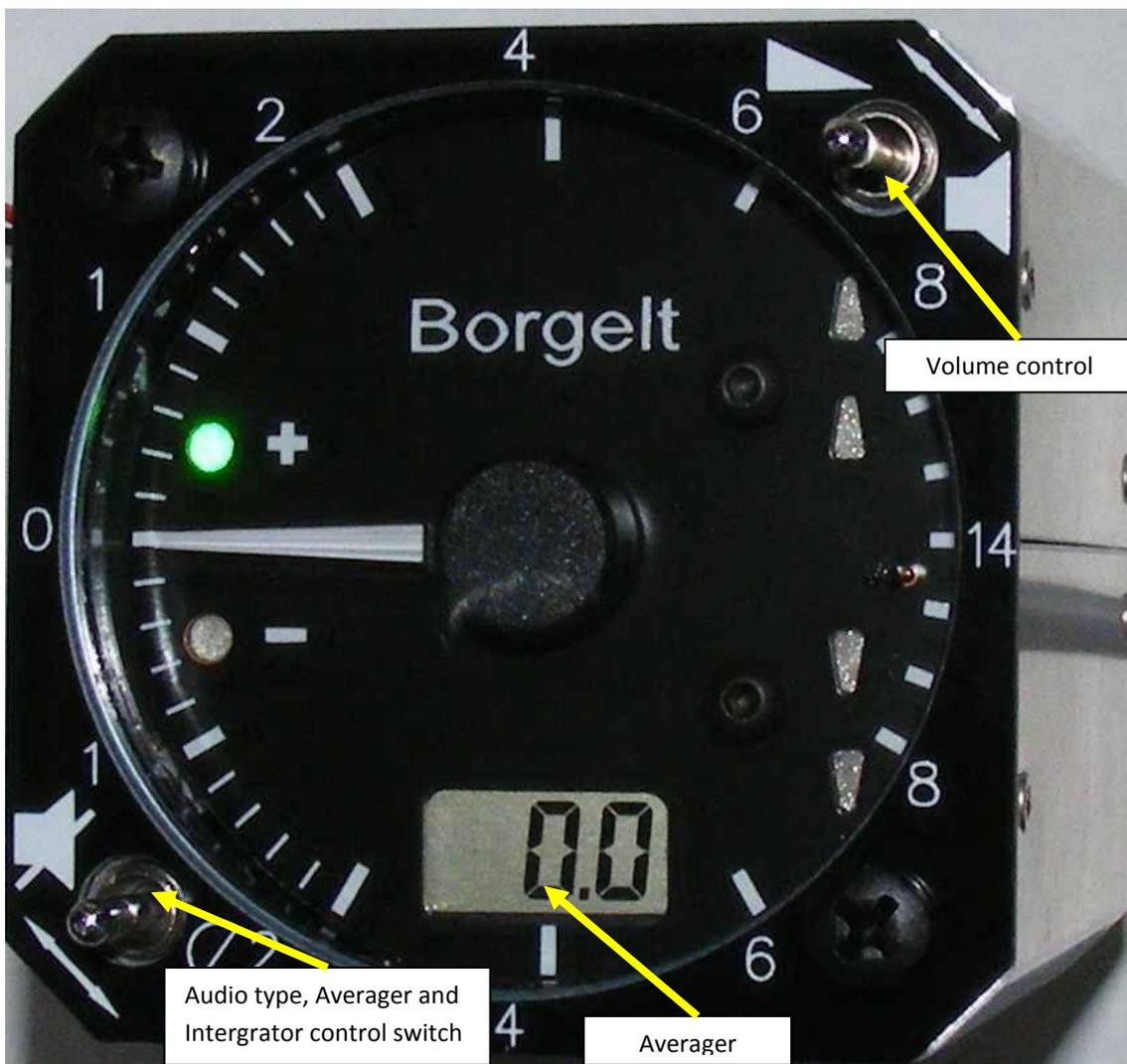
The Borgelt B700 is a standard T.E. vario with inbuilt digital averager readout and battery backup to supply power to the unit incase of instrument power loss. The dial is a non-linear type that makes the vario pointer very sensitive between 0-2knots, less sensitive between 2-8knots and even less sensitive between 8-14knots.
