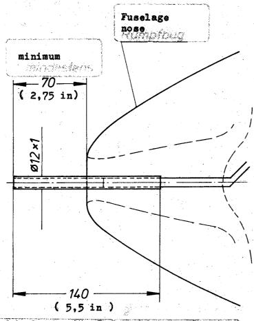
Extension tube for total pressure head with inverted flight. Brass tube 140 mm
