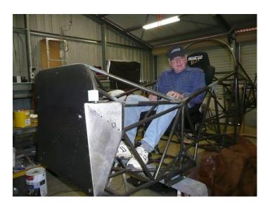
The fuselage frame is now substantially complete. Seat, firewall and elevator circuit are fabricated and installed (Installed for the rirst time, as everything has to come apart again for painting, before fabric is applied) The aileron bell crank is fabricated and ready for installation. I am waiting on the drawings for the aileron push rods.
